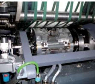
Cylinder stitcher integrated in the folder with double circumference and dedicated AC motor drive (11 millimeters and/or 16 millimeters staple sizes).
